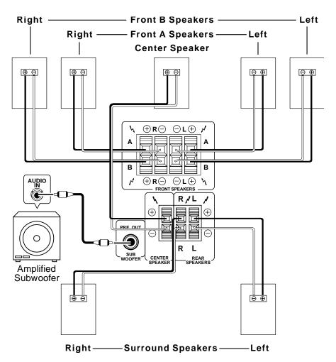
**Note:** Be sure you connect the receiver's right and left positive (+) and negative (-) terminals to the speaker's corresponding right and left positive (+) and negative (-) terminals.
